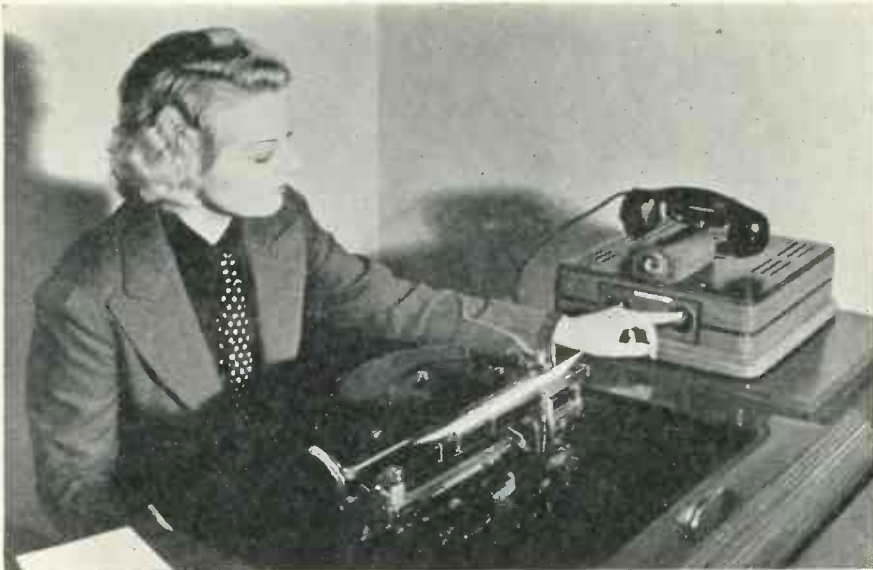
New multi-station system by Carrier-Call allows user to select any one of 5 other stations, talk without others hearing. "Carrier-Eye" used for busy signal.
